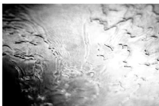
Fig. 1 Surface waves on a smooth rotating disc surface.
